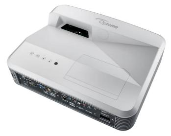
It provides a complete package for engaging learning with many new features, including two HDMI inputs, powered USB port, powerful 16W built-in speaker, improved lamp life, compact chassis and a completely new mounting system for a fast and simple setup.
