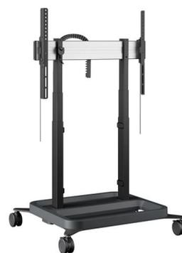
The RISE 5305 motorised display lift trolley is suitable for displays of up to 86" with a maximum weight of 120 kg. The lift raises the display smoothly, quickly, and safely at a speed of 50mm/s with QuickRise™. With a 980mm travel range the lift is suitable for both very low and high positions.
